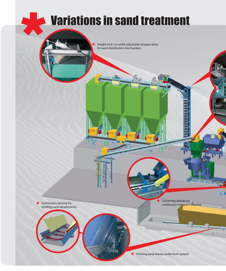
Sand treatment systems for steel casting, nodular graphite casting or aluminium casting are optimally planned and projected. Our own production, "Made in Hörstel", guarantees continuous quality and stable operational safety. Service and assembly performed by VHV mechanics ensure timely commissioning of the foundry systems.
