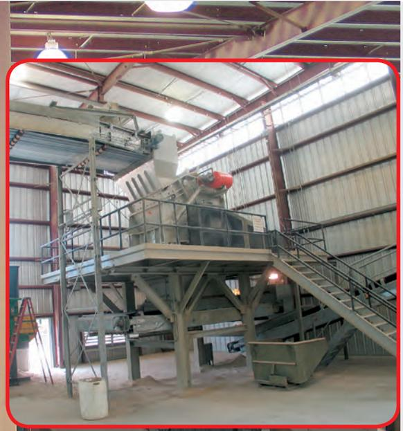
\* Belt conveyor before and after the crusher
