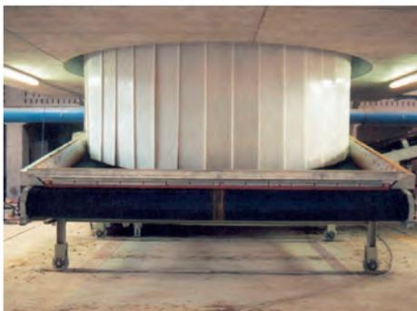
\* Up to 5.200 mm belt width below the pan mill
