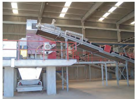
\* Hinged belt conveyor with material distributor as well as intake and discharge chute
