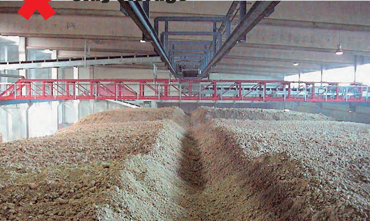
\* Clay storage with shuttle conveyor platform
