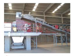
Hinged belt conveyor with material distributor as well as intake and discharge chute
