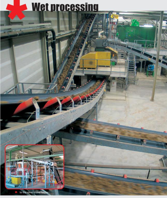
\* Conveying for grinding, rolling and mixing
