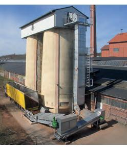
★ Double belt conveyor for filling the clay silo
