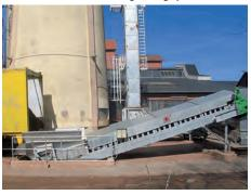
Truck acceptance belt conveyor, belt width 2000 mm
