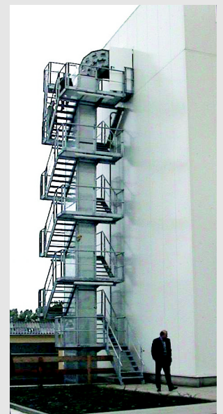
VHV double belt vertical conveyor with a stairs tower
