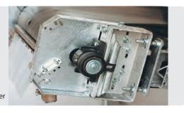
Drive station with back stop and front segment scraper
