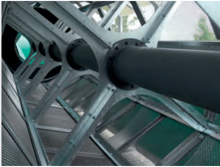
* Torsion resistant, inclined screen body (internal view)
