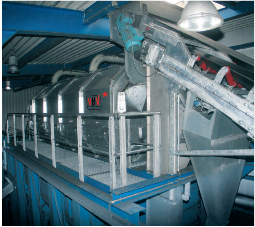
* Iron elimination through magnetic drum with discharge shafts for iron and trickling sand.
