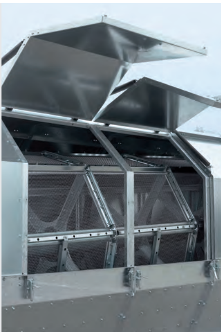
* Trouble free maintenance through easily accessible, pre-stressed screen areas of similar construction.
