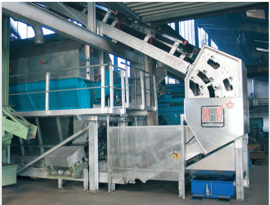
* The VHV belt conveyor outlet enables the installation of the polygon screen at ground floor level or in basements.
