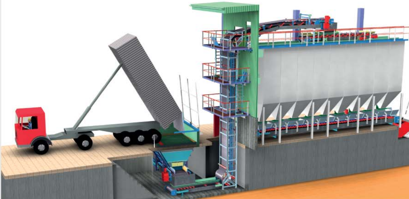
* Purified silo feed with truck receiving, double belt conveyor, reversible shuttle conveyor, dosing hopper and weighing belt.
