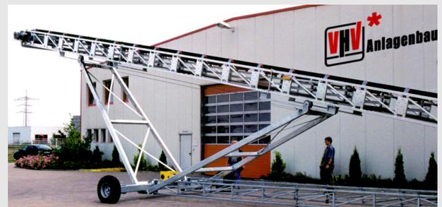
*swivelling undercarriage adjustable in height*
