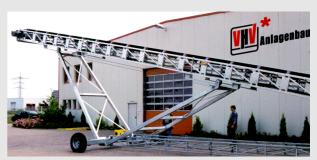
swivelling undercarriage adjustable in height
