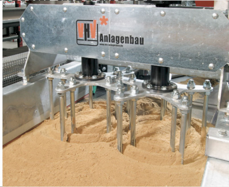
Hinged without having to disassemble the mixer plates
