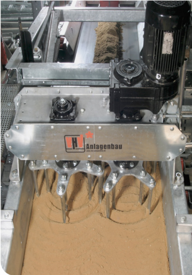
Hinged without having to disassemble the mixer plates
