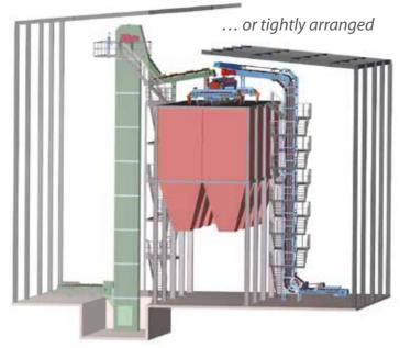
**VHV's double belt conveyor** replaces: The infeed belt, bucket elevator, connecting conveyor, stair tower, basement deepening as well as the raise of the roof.
