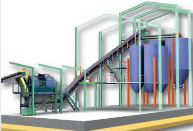
* Cover belt conveyor between polygonal sieve and silo
